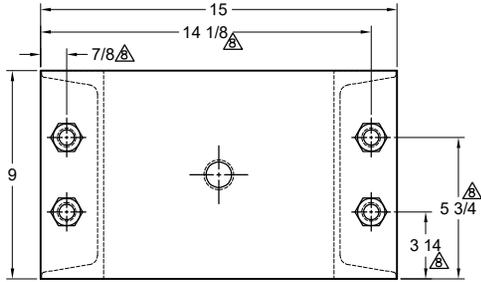
**TYPE ME-4D SPRING ISOLATORS WITH INTERNAL ADJUSTMENT**
